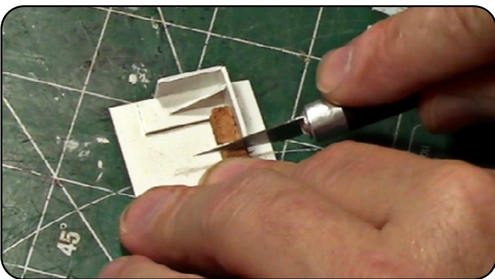
Push the cork strip up to the stop and cut with a sharp hobby knife blade.
