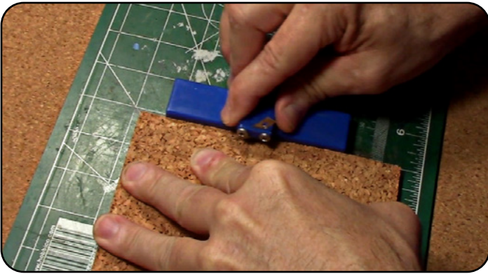
Use a balsa stripper to cut perfectly-straight lengthwise cuts.
