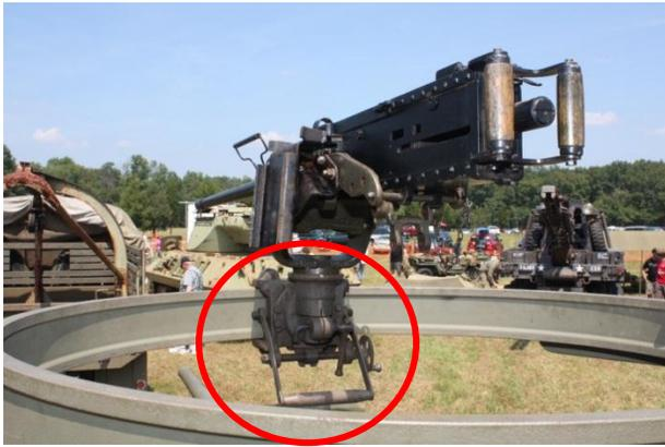
Figure 11, MG traverse mechanism
