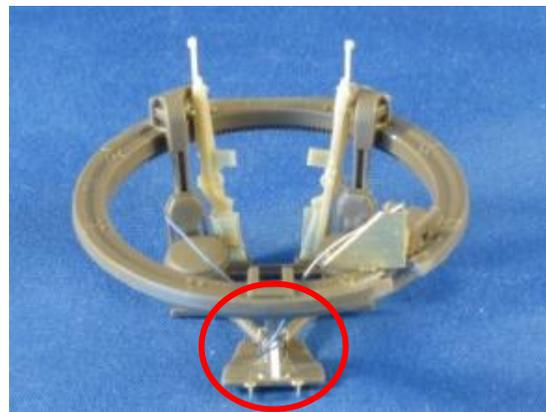
Figure 10, Floor plate trigger assemblies
